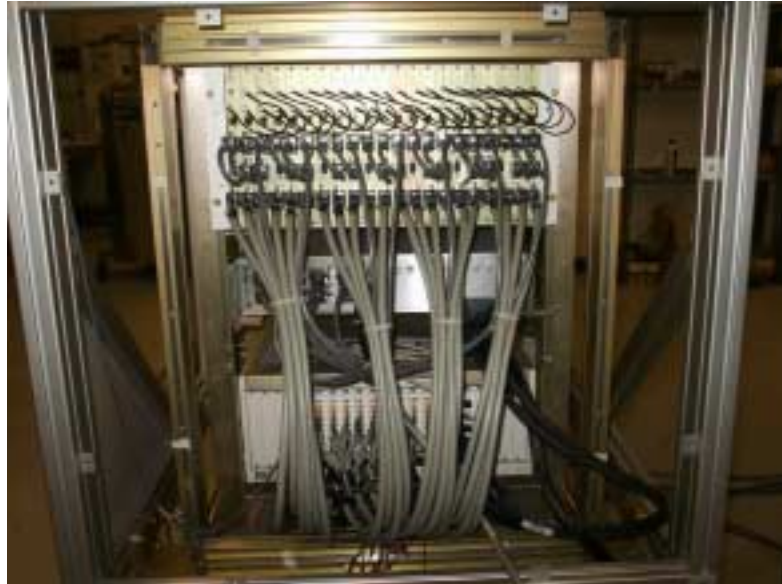
Figure 2: 84 channels of iMAG400 electronics in a standard rack mount card cage. The power distribution hub is located in the middle of the rack. The lower electronics box contains 84 channels of 24 bit data acquisition cards.
