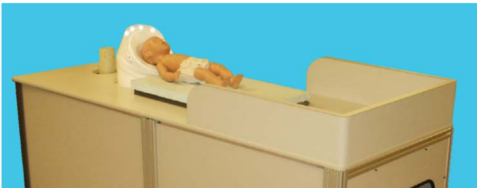
Figure 1. Realistic size dummy of infant shown on cart with sensor cradle.
